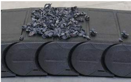
Example: Cover system with chips
